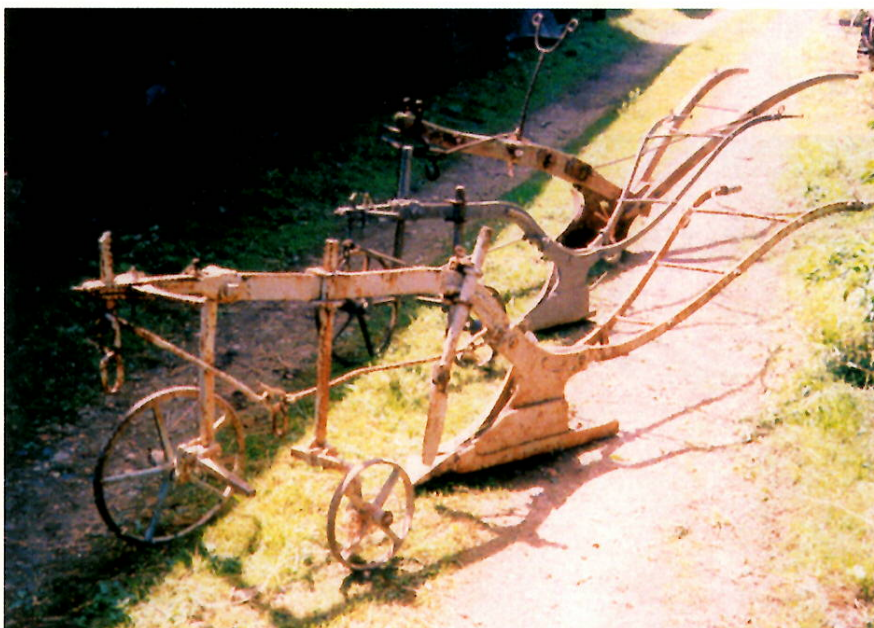
A trio of Cannings ploughs: from front to back, a long-framed and ley-bodied No. 5, a more compact digger-bodied model XL and the little wood and iron L2, once so popular with local market-gardeners and smallholders.
