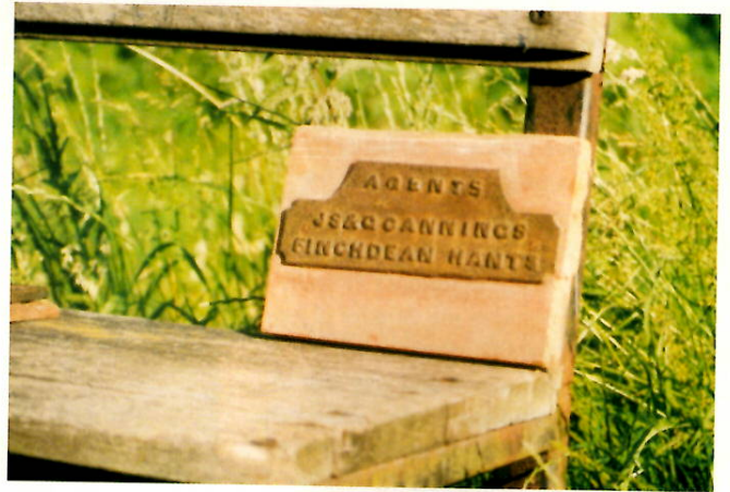
Cannings' agent's plate cast in their works for fitting to the other manufacturers' products which they sold. This one was probably from the feed-box of a chaff cutter.
