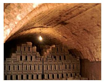
When the firing of the bricks was completed, the kiln chamber was allowed to cool down for two or three days. The entrance (wicket) door was broken down to allow further cooling. Once the temperature had dropped enough, the process of removing the bricks got underway.
